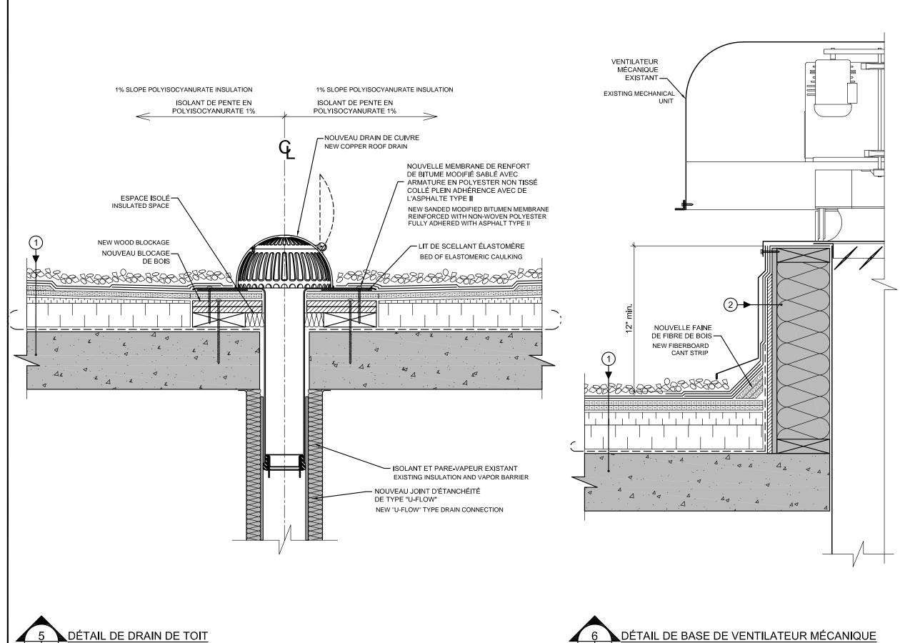
**ROOF DRAIN DETAIL**
