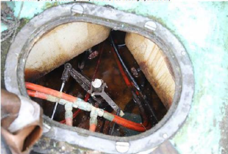
Image 4: Montego Bay (Steering Compartment, free floating hydraulic oil)
