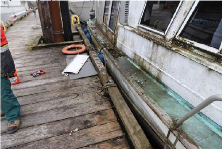
Image 2 : Montego Bay (Starboard side, rotten deck area)
