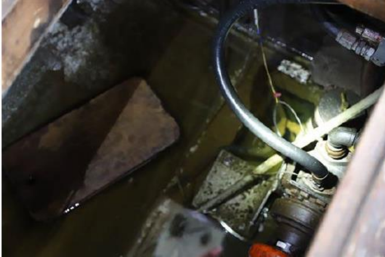
Image 3 : Tanner's Quest (Steering Gear, sludge)
