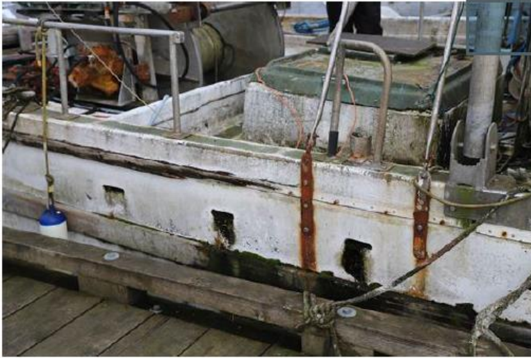
Image 4: Tanner's Quest (Port Side, some hull deterioration)
