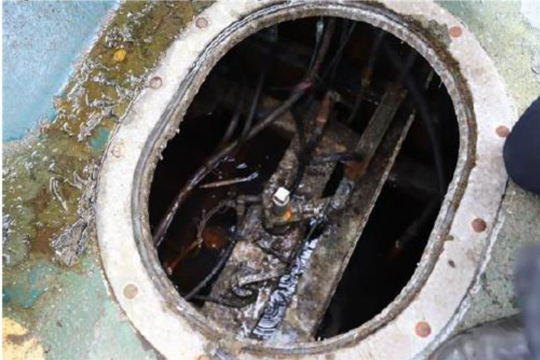
Image 3 : Tanner's Quest (Steering Gear, sludge)
