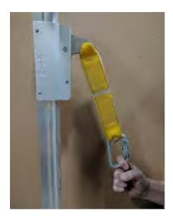
**Step 3:**To ensure Trolley is functioning properly, pull down on karabiner to duplicate a fall arresting situation. Trolley should grab safety rail immediately.
