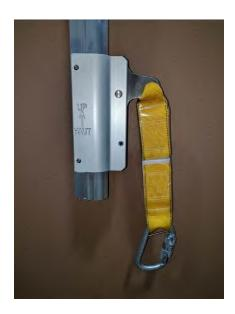
**Step 1:** Hold the Trolley so that the UP arrow is pointing upwards and insert trolley onto bottom of rail.
