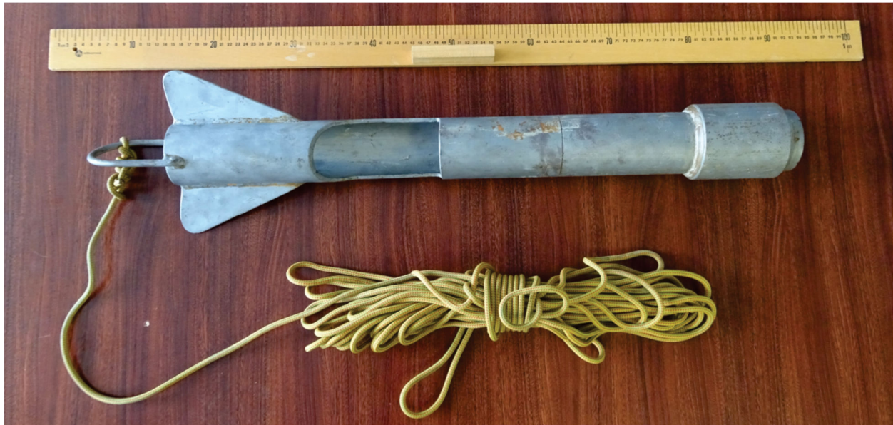
Figure 1. Lake sediment sampler used at the Geological Survey of Canada. The device weighs 7.1 kg and collects a 30 cm core sample of lake sediment, corresponding to a weight of 1.2 kg of lake sediment.
