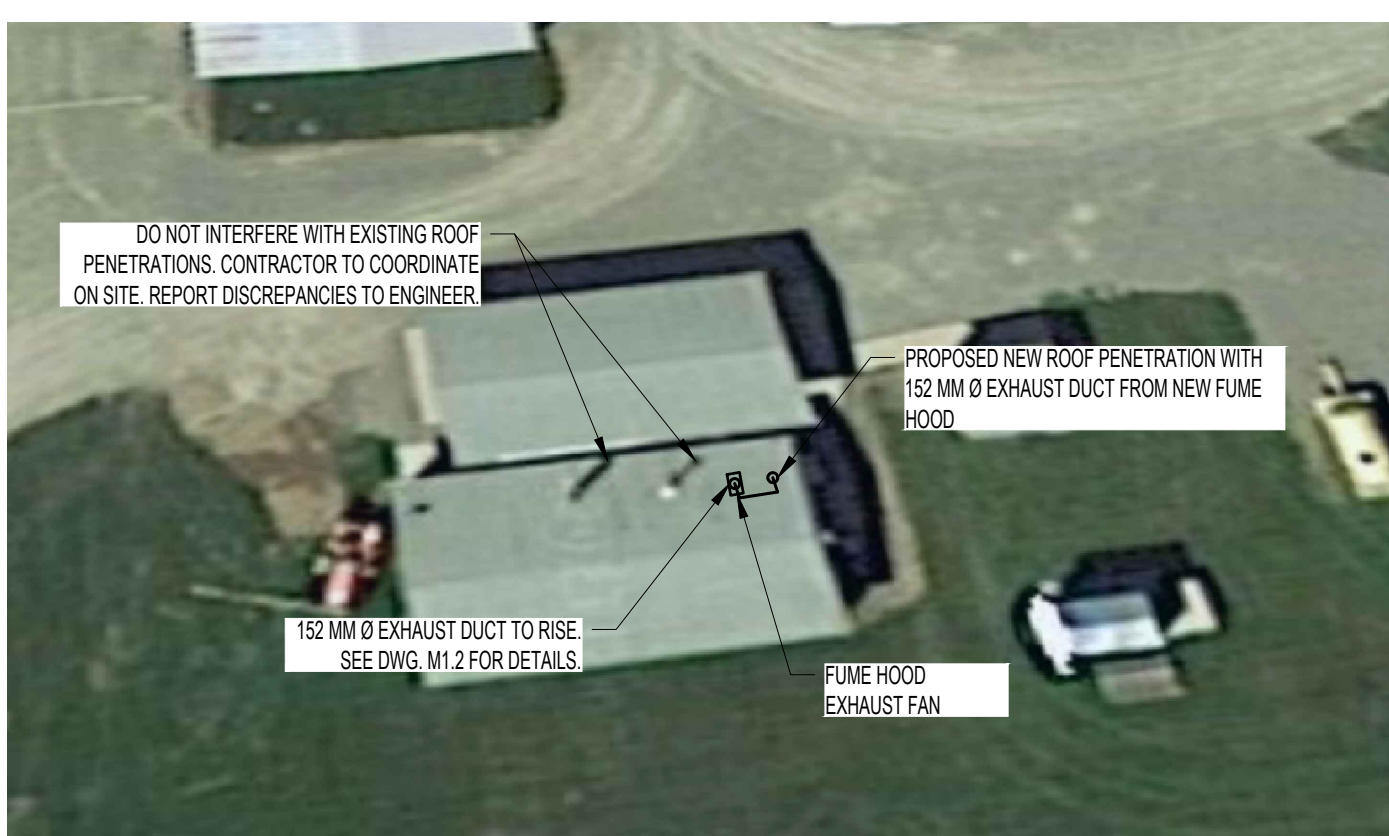
IMAGE #1: ROOF PENETRATIONS
